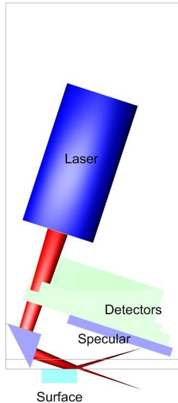
8826 can “over-illuminate” a small surface and measure roughness
