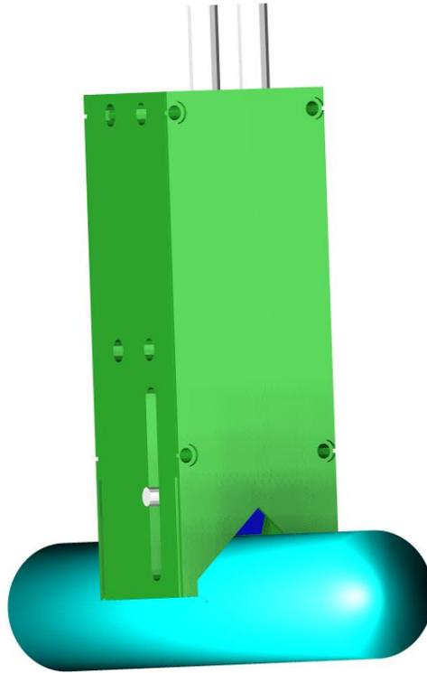
8826 on Cylinder Surface with Alignment Fixture Setting Correct Horizontal Position
