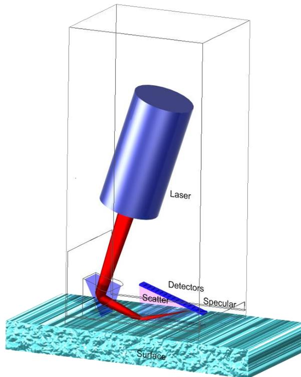
Schematic Diagram of Lasercheck Instrument
