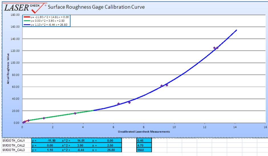
Calibration graph from Lasercheck Calibration Spreadsheet
