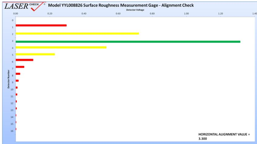
Typical Spreadsheet Alignment Curve Showing Specular on Detector 3
